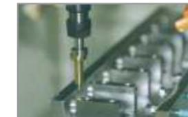
2. When measuring probe touches workpiece, it looks in "one part."
