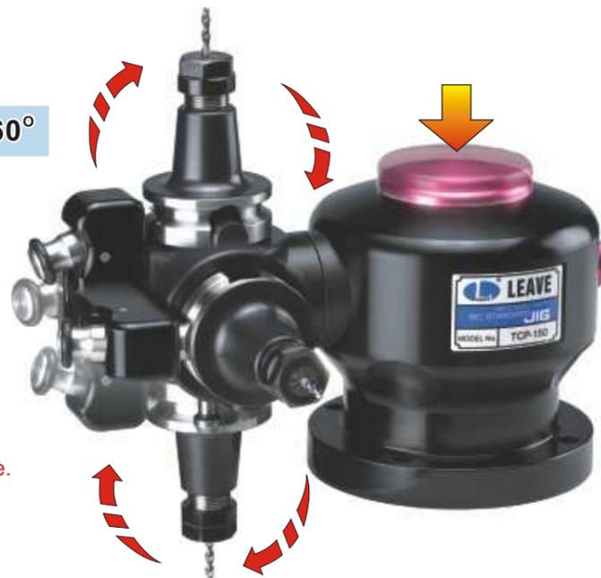
4pcs of M10x40mm bolt can be fastened from the top of the mounting flange or 4pcs of M12 bolt can be fastened from the bottom of the mounting flange.
